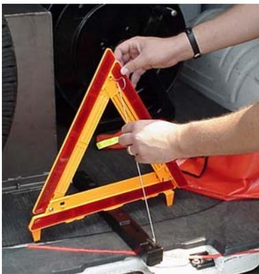
Once the triangle has been assembled, it should be turned on the base to provide better stability. Raise the metal rod, squeeze together, and slide into the hole at the top of the triangle. Under normal conditions, the weighted base will prevent the triangle from tipping over.
